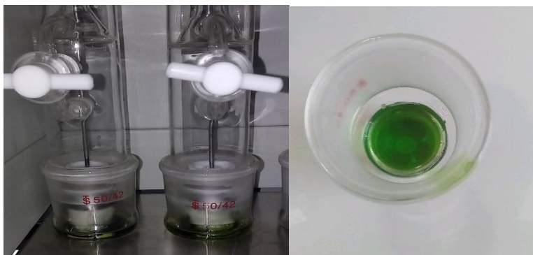
2-rasm. Oddiy tog'rayhon ( Origanum vulgare ) o'simligidan sokslet apparati yordamida efir moyi ajratib olish jarayoni.
