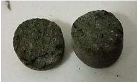
Figure 2. Clinker fired at 1380 °C from the raw material mixture of JSC “Bekobodsement”
