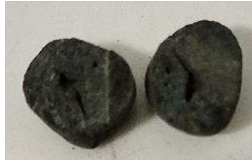
Figure 3. Clinker fired at 1380 °C from the experimental raw material mixture
